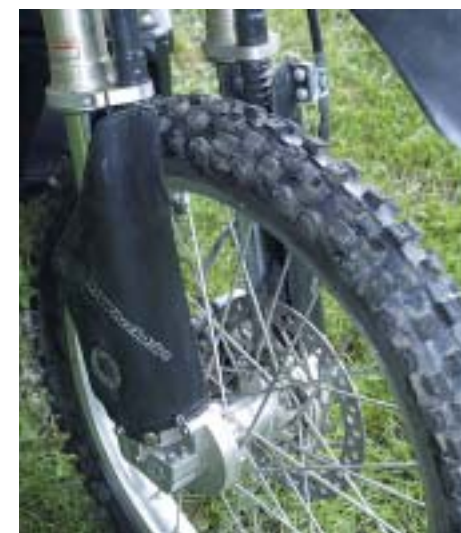
Power is transmitted by twin telescoping shafts down the front of the forks. The stock axle carriers on the lower forks were replaced with a pair of drive mechanisms to power the stock Honda hub.
