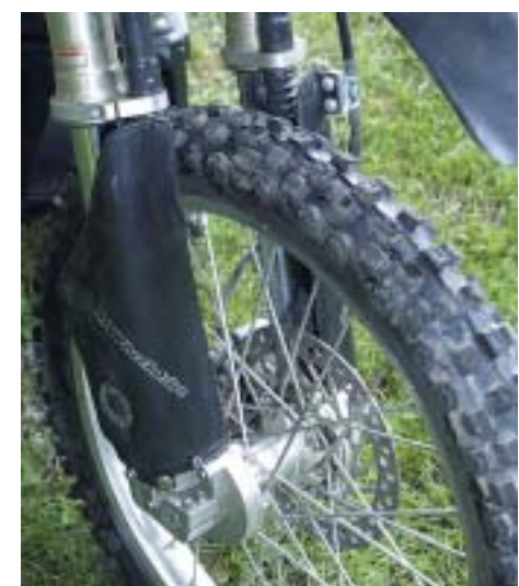
Power is transmitted by twin telescoping shafts down the front of the forks. The stock axle carriers on the lower forks were replaced with a pair of drive mechanisms to power the stock Honda hub.
