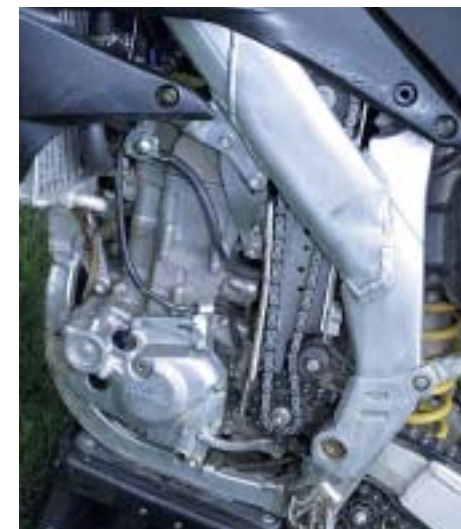
A small sprocket on top of the countershaft sprocket transfers power to the steering head, where it is turned and pointed at the front wheel.
