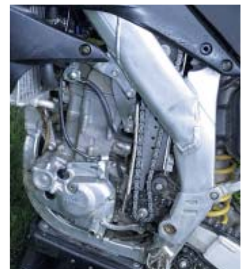
A small sprocket on top of the countershaft sprocket transfers power to the steering head, where it is turned and pointed at the front wheel.
