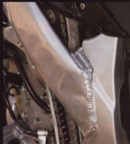
The left-side frame rail is pushed out a bit to make room for the chain. The bike scaled in at nearly 30 pounds more than a CRF450R, but more than one experienced test rider guessed it was only 15 pounds heavier—a testament to the way 2WD makes a bike feel more active and lighter.
