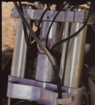
Not to be goony but to show off the product, Christini runs no front number plate to let you see the oversize head tube/gearbox. It and the lower triple clamp are the key components to the patent.
