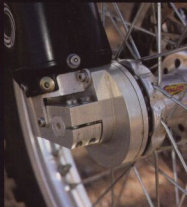
Trick fork lowers house a gear set and transfer power to a Talon hub with a one-way clutch. The wheel is only slightly harder to remove from the bike.
